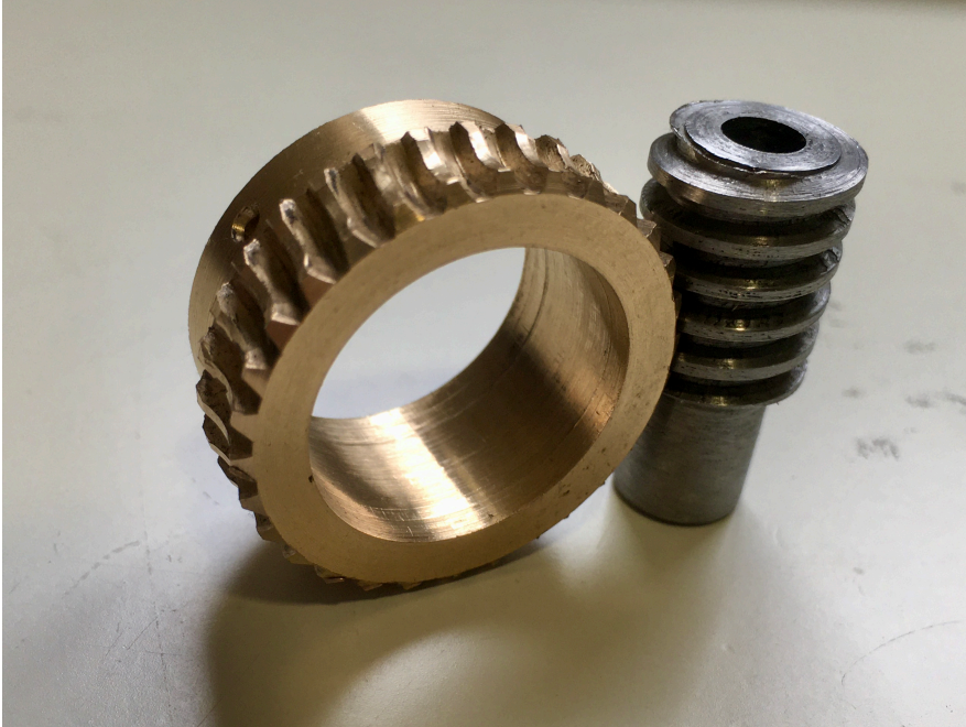
30 tooth phosphor bronze worm gear and steel worm cut with an Acme profile.
