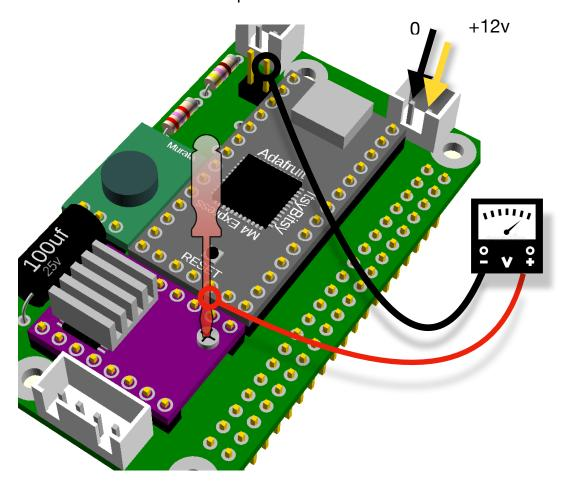
Set the multimeter to read DC volts and touch the screwdriver (connected to the positive terminal) to the adjustment screw indicated by the screwdriver on the graphic. Turn the screw whilst reading the meter until the voltage is equal to half the current rating of the motor windings.
