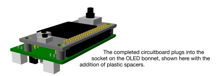
The circuit assembly is mounted with 4 screws to a plastic face plate which in turn fixes to the steel mechanical assembly. The buttons have been extended with a plastic component.
