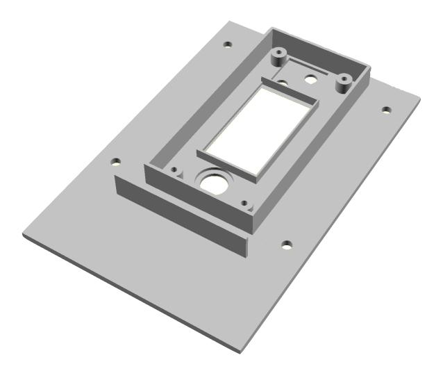
As the buttons on the OLED display are very short it is necessary to extend them. This plastic item does the trick. And as they are joined together, easy to handle. The base is made very thin so as to remain flexible. This ensures that the buttons don't interact with each other when pressed.
