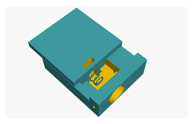
As the X and Y slides need to operate in tandem they must be stuck together at right-angles to each other. I was planning to use superglue but in the end used thin double sided tape which proved perfect for the job and offered the opportunity of disassembly should mistakes be made. Consider the final orientation of the micrometers when sticking the two slides together.
