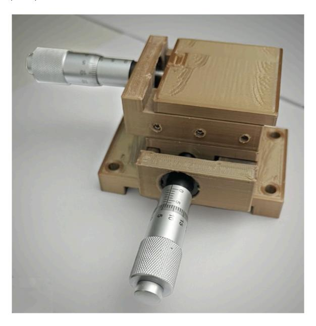
The micrometers are graduated to 0.01mm but given all the vagaries of the construction an accuracy of +/-0.01mm is probably more realistic which in English is better than a thousandths of an inch.
