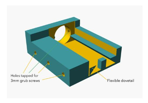
Here the fixed slide is shown with its grub screws and plugs.
